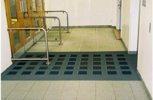
This new Nomad modular matting system combines high performance with flexible design options and easy on site installation. This matting system is made up of two tile versions, each incorporating a 2mm drainage foot on the bottom surface. The large open scraper profiles incorporate 'heel steps' to prevent heel trapping. Traffic rated at 5000 crossings per day
